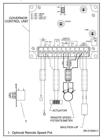
Figure 6-26 Remote Speed Adjustment
